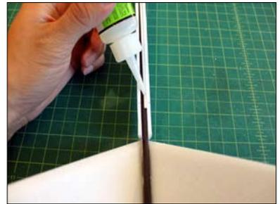
Apply glue all the way up the tail boom with the pushrod tube inside.
