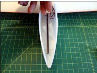
Take the larger of the 2 pieces (5 part stack) and insert it in the fuselage with the groove facing up.
