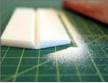
Use a sanding block and sand an even taper along the trailing edge.
