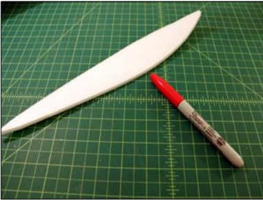
Again using the marker curve the canopy to match the shape of the fuselage
