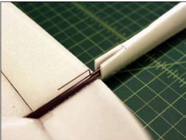
Insert it from the tail up. Line up the raised part of the push rod to stand up.
