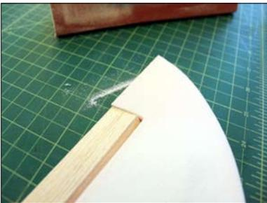
**OPTIONAL:** Flip over the wing and sand the bottom trailing edge wing tip. This will create some slight washout.
