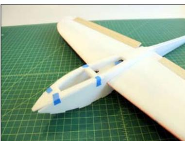
For now don't glue the top. Just tape it down to hold the shape while we glue the bottom on.
