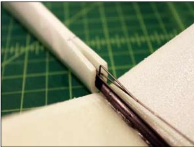
Lay down the shorter pushrods into the channel where the pushrod tube is.
