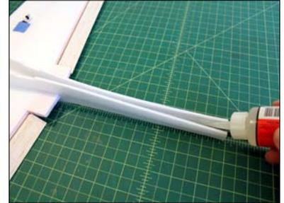
Attach the sides all the way up to the trailing edge of the main wing. Do not glue above the wing. You should only glue down the carbon tail boom.
