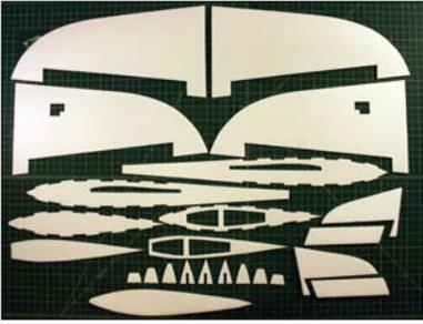
Cut out the foam parts from the sheets by trimming the tabs. You should be left with these parts shown.
