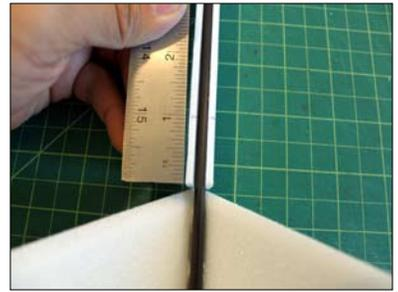
Insert your pushrod tube into the groove on the top of the fuselage boom.
