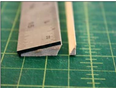
Using a metal ruler you can trim off about 30 degrees to created a bevelled edge. If you prefer you can simply sand it instead of cutting it as shown.
