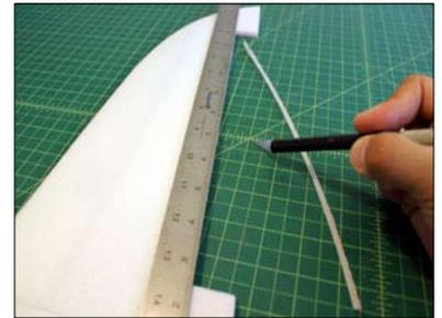
Lightly sand if needed. This is the top view of the wing. Bevel the edge about 30 degrees Bevel it so the sharp edge is on the top of the wing.
