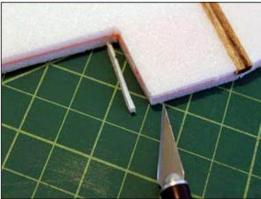
Check both sides of the aileron cut out of each wing both top and bottom. Again, trim if needed...
