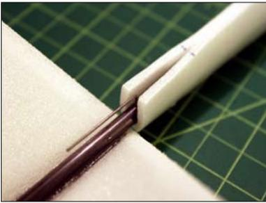
Make sure the pushrod is still standing up with locking down the Ez-connector.
