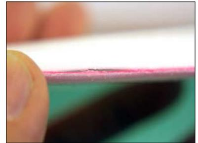
After some glue and a spray of accelerator an you can not notice any crack.
