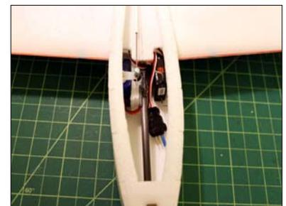
Flip over your glider and install the aileron control linkages. Mark the location for your control horn at 1/4" from the hinge line.
