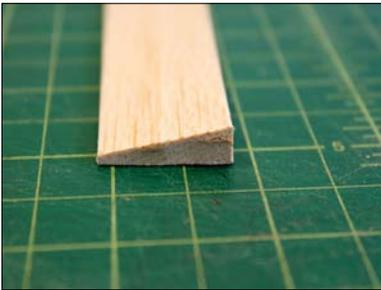
Locate the correct position for the balsa ailerons. You will see that only 1 corner is a 90 degree corner. That side is the bottom.
