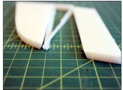
You should have an upside-down V groove when you line up the elevator on the stabilizer.
