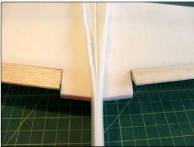
Close it up to the end of the trailing edge. Do not glue above the wing. Just close up the tail boom.
