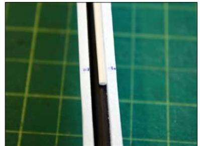
Apply glue above the 1" inch mark. Don't let any glue drip down to the end of the pushrod tube and clog up the hole.
