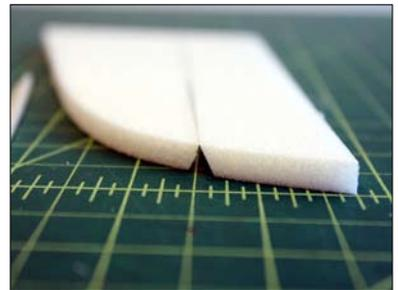
Tape both elevators together so we can sand a tapered trailing edge on each elevator and have something to grab onto while sanding.
