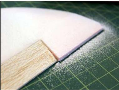
Sand the wing tips to closely match the taper of the aileron. Don't over do it since you will also sand the bottom. Here you can see the red marks showing through to gauge your sanding.
