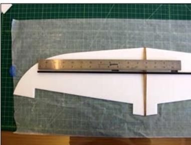
Lay out the carbon fiber tube in the slot of the wing rib. Center the carbon tube 12" inches to each side of the rib.
