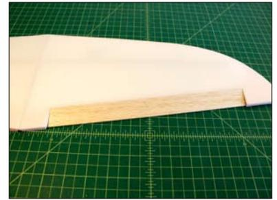
Again, using a metal ruler trim the wing to create a bevel where the aileron will attach. We will be bevelling BOTH the aileron and the wing.
