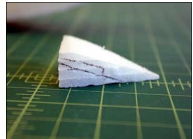
Cut it off with a straight cut. Again do not cut the stepped line.
