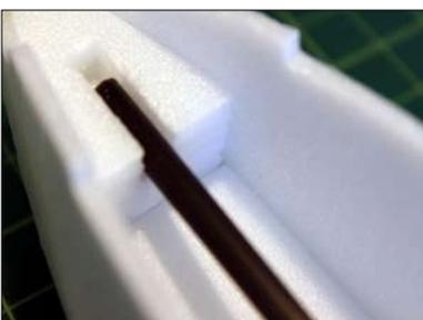
Slide it all the way forward until the carbon tube pops into the groove as well as the opening on bottom sheet.
