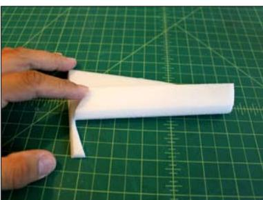
Flip up the elevator and tape the under side.
