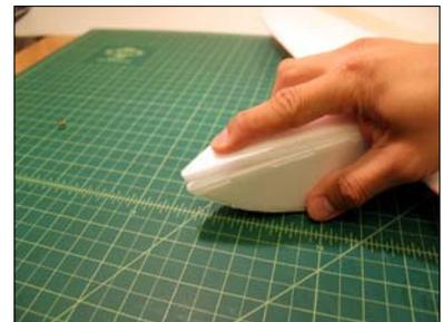
The underside of the canopy shows the impression to cut out the hole.
