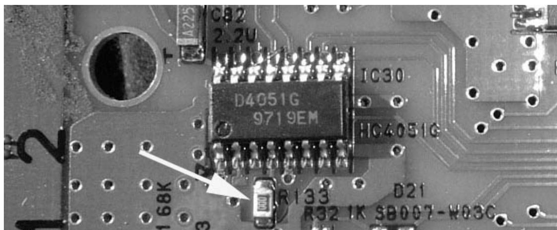
No.Resistor (open circuit) = stick mode 1, T9ZHP (heli)
