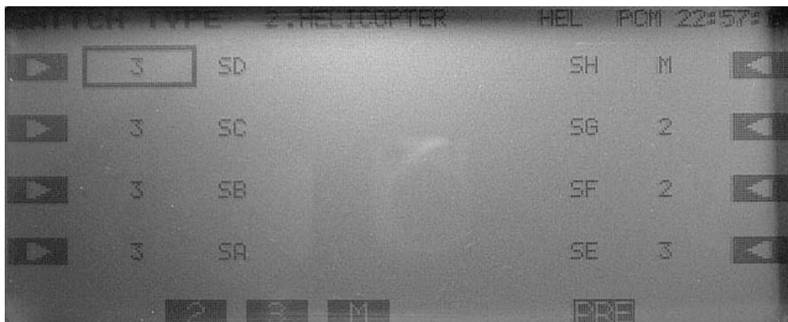
This screen allows customization of the switch configuration. Obviously physical replacement of the switch is also required. All types of switches have the same number of contacts and identical footprint which makes direct replacement possible.
