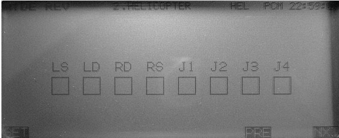
Move both sticks fully right and fully down, set knobs fully clockwise and sliders fully down. Press [SET]
