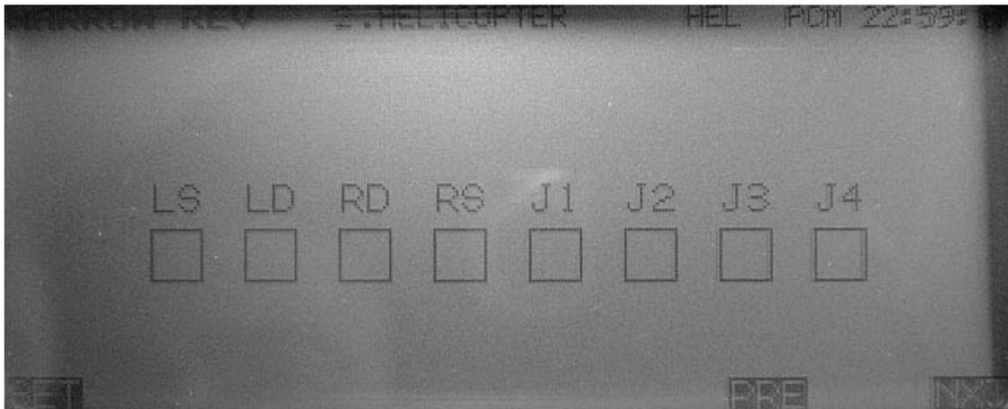
Move both sticks fully left and fully up, set knobs fully anticlockwise and sliders fully up. Press [SET]
