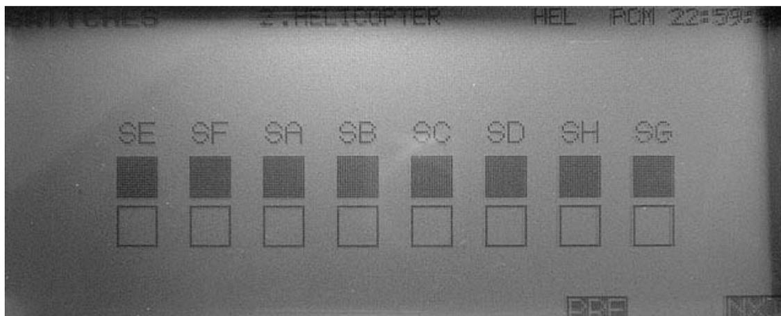
Toggle switch check. Move switches to all position.
