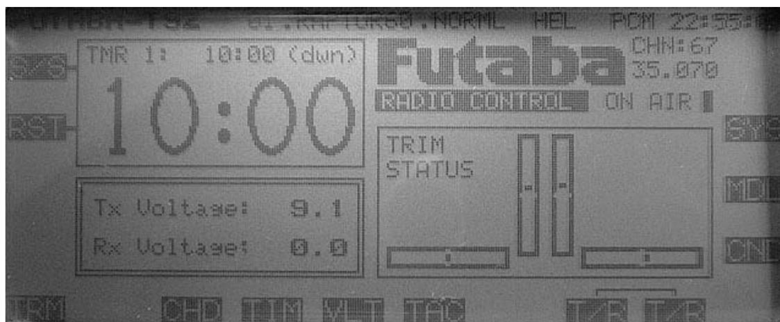
Most Futaba radios have a formerly secret service menu implemented into their firmware. This menu was designed for transmitter testing and servicing, but also allows a degree of radio customization.
