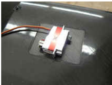
Servo locations have the skin indented for covers. Your kit may have the servo wells already made at the factory. If so, you can skip a few steps.
