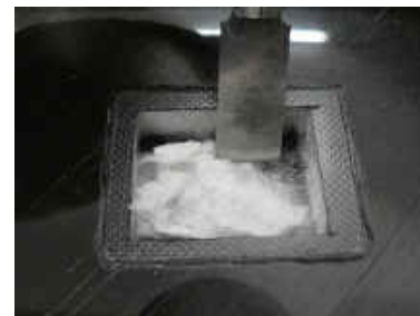
Pick out the foam inside the servo pockets carefully, first with a regular X-acto knife, then using a spade knife when near the top skin.
