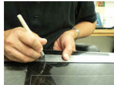
Start by cutting out the skin inside the servo locations.
