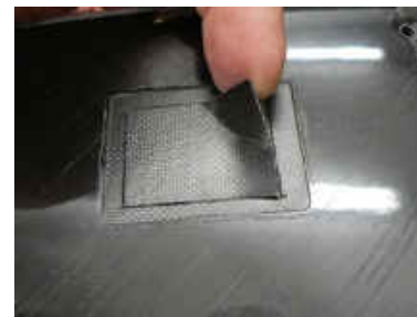
Peel off the skin carefully. The cuts should be at least 3mm inside the outline. More if your servo is smaller and you want to reduce the size of the servo pocket.
