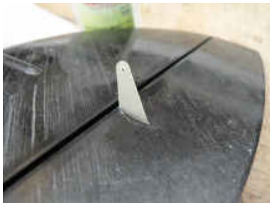
Rudder control horn installed similarly. No slit is necessary since the control cable will be attached permanently.
