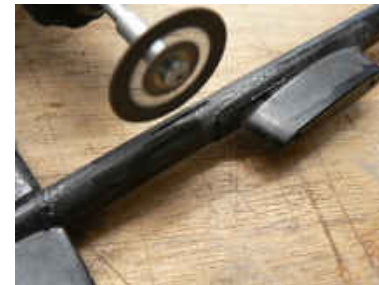
Make slits in the tail boom for cable exits. One for the rudder cable, behind the stab mount, and one for the elevator cable on the opposite side, in front of the stab mount.
