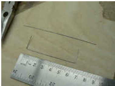
Make two torsion springs for the rudder and the elevator from the supplied 0.5mm spring wire.
