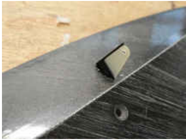
Elevator control horn installed with CA.
