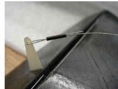
Insert the rudder cable into the slit and run it all the way to the front. Insert the rear end of the cable into the rudder control horn, make a loop, and crimp the cable with a small piece of copper or steel tube. Squeeze the tube with pliers to create a permanent crimp.
