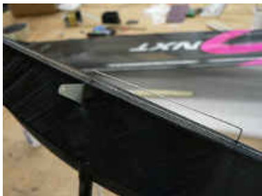
Make two holes, one in the rudder near the control horn, one in the main part of the vertical tail, using either a micro drill bit or a sharpened piece of slightly thicker wire. Insert the U-spring into the holes. Apply a tiny drop of CA to each hole to reinforce the foam and lock the spring in place.
