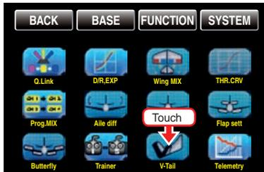
The elevator and rudder are controlled by two separately-actuated rudders arranged in a V-shape. The coupling function for the rudder and elevator control is automatically transferred from the program.
