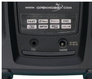
The charging socket comes standard with a protective diode that protects against polarity reversal. Original *Graupner* automatic chargers recognize the battery charge. Note the setting instructions of the charger which is used.
