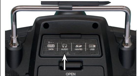
The socket is for connecting commercially available earbuds or headphones with a 3.5 mm stereo jack (not included in the set). When headphones are plugged in, the transmitter's speaker is switched off, and the stylized icon of a headphone is depicted in colour and not grey in the basic display, see page 20.
