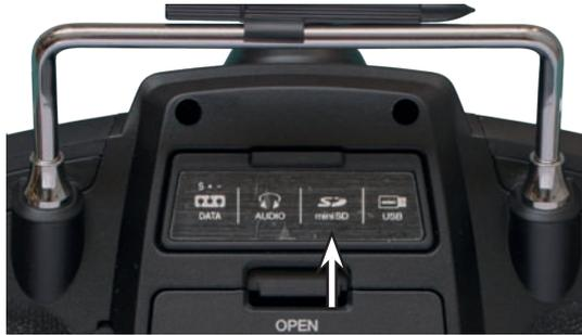
In addition to the micro-SD memory cards that come standard, all conventional micro-SD memory cards with up to 2 GB and micro-SDHC cards with up to 32 GB memory can be used. The manufacturer recommends using memory cards with a maximum of 4 GB since this capacity is normally sufficient.
