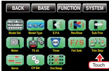
The two control sticks come with digital trimming. With each click, briefly touching the trimming lever, moves the initial position of the control stick by a certain value. If it is held, the trimming moves in the corresponding direction with increasing speed.
