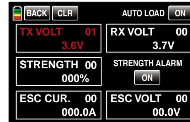
... depending on the selected battery type in the line above, in increments of 0.1V between 4.5 and 5.5V (NiMH battery) or 3.4 and 4.2V (lithium-ion/lithium polymer battery). Make sure that the set value is not too low to give you sufficient time to land your model after a battery warning.
