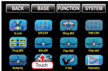
An aileron deflected downward generates greater resistance for aerodynamic reasons than one deflected upward.
