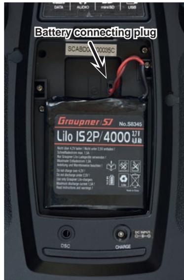
Then disconnect the transmitter battery plug by carefully pulling the supply cable. Then lift the battery and pull it gently off of the velcro.
