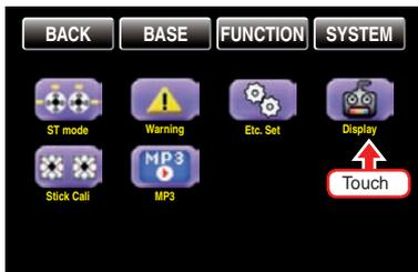
In the "Display" submenu, you can enter display settings such as changing the contrast, turning the backlighting on or off, and adjusting the touch sensitivity to your preferences. Furthermore, you can change the color of the transmitter logo, and switch on and off a function that makes it easier to read the display in a sunny environment.
