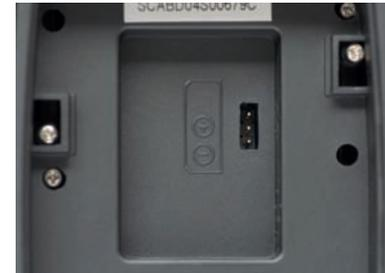
Never forcefully insert the plug into the socket on the transmitter board.
