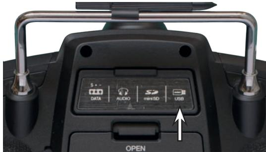
The USB cable that comes with the set is plugged into this socket. The procedure for obtaining software updates through a computer is described in the software package instructions.
