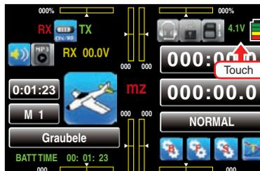
*... the voltage display and hence the threshold of the battery warning can be fine-tuned using a precision voltmeter.*
