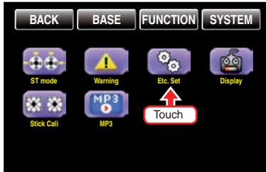
In the submenu "Etc.Set", you can switch on and off the defaults for the lines "Battery type" and "Batt warning", as well as the volume of the acoustic output and the power-on melody of the transmitter.
