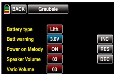
Touch **INC** or **DEC** at the right edge of the display to select the appropriate warning threshold, for example:
