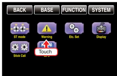
In this submenu, you can switch on and off five triggers of a visual and acoustical alarm. Normally, only the throttle/pitch control stick is actively monitored. The options "Throttle hold", "Throttle Cut", "Quick Link" and "Power OFF time" can also be activated.
