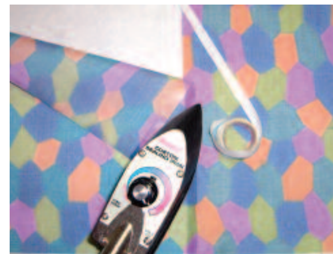
Use the covering iron to bond the printed fabric panels together.
