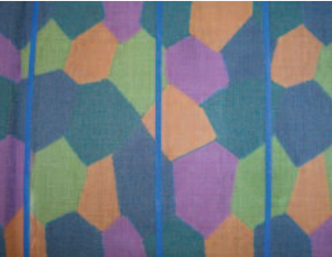
This close-up of the finished wing shows how real the fabric weave looks on the model. The blue rib tapes were added after the fabric had been shrunk tight.
