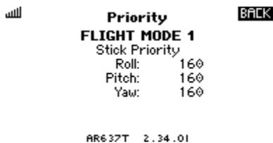
If you have configured the Gain Channel, then you can select which axes would be affected by making adjustment during flight on the "Fixed/Adjustable Gain" screen.
