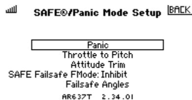
The settings in Section 2 assigned the panic control channel to be Aux 2. I also adjusted the envelope limits to be a lot tighter, especially for pitch (nose) down. You also need to select a flight mode that Panic should use for gain settings. Select the flight mode that has self-level enabled.
