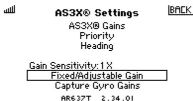
When set to "Fixed", the Gain Channel adjustment would be ignored by that axis. The default setting for all AS3X Gains is "Adjustable".
