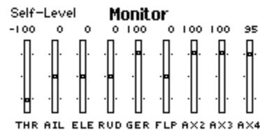
The AIL, ELE, and RUD channels will move with the sticks. Go ahead and play with it. **BE CAREFUL WITH THE THROTTLE IF THE PROPELLER IS MOUNTED ON THE PLANE!**
