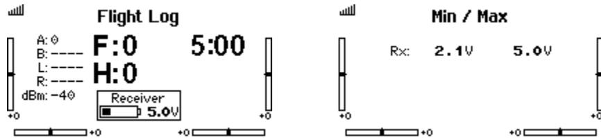
You can turn on the collection and display of additional telemetry information from the built-in sensors on the receiver. To do this, go to the Function menu, and then Telemetry.
