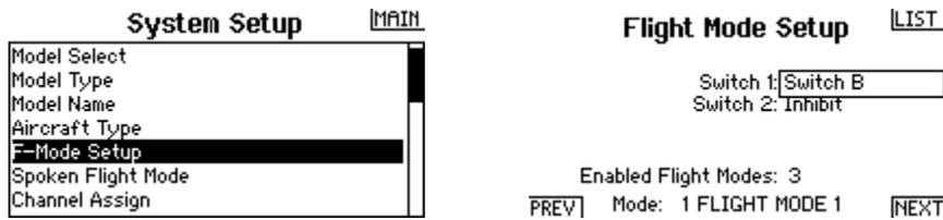
At the bottom of the screen, you should see that there are three enabled flight modes. You can even test it. If you flip Switch B through its positions, you should see the text change at the bottom of the screen.
