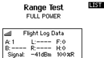
You'll see the signal strength level at the bottom in both dBm (the technical measurement) and a percentage. The dBm reading should be somewhere between -40 dBm (about as good as it gets) and -85 dBm. Anything worse than -85 dBm would be considered poor reception.
