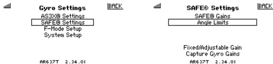
That will take you a screen where you can adjust the angle limits for each flight mode by flipping the flight mode switch.
