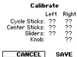
On this screen, move the sticks in the shape of PLUS SIGNS, not circles. Move each stick up and down, back to center, and then left to right. Repeat the movement a couple of times until the screen shows "OK" instead of "??". For knob and slider inputs, move the input all the way from one end of its range of movement to the other. When all items are "OK" select "SAVE" to save the calibration.
