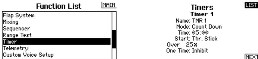
Change the time to a value that’s appropriate for your model and flying habits. If you’re not sure which value to use, consult the manual for your model. Note that it is not good for the batteries to keep flying until the motor reaches the Low Voltage Cutoff warning. You want to land before that happens! Over time you’ll find the optimum setting for the timer based on your flying habits.
