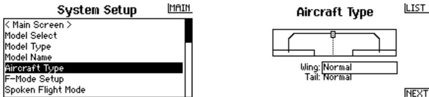
For a plane with simple controls for elevator, aileron, and rudder, leave the Wing and Tail set to Normal.
