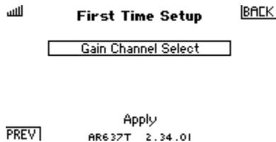
Going into that screen displays which switches are currently assigned to each channel, and then ask you for a Gain Channel input. If you’d like to take advantage of this feature, you would assign a channel for that purpose here (as shown). There will be more on how to use this feature later, but for now I’m going to go ahead and assign Aux3 (the knob) to this function.
