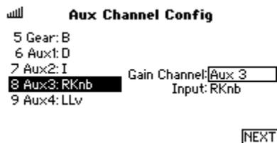
At this point it has enough information for the basic configuration of the receiver. You can choose “Apply” to apply the settings, and then it will update the receiver.
